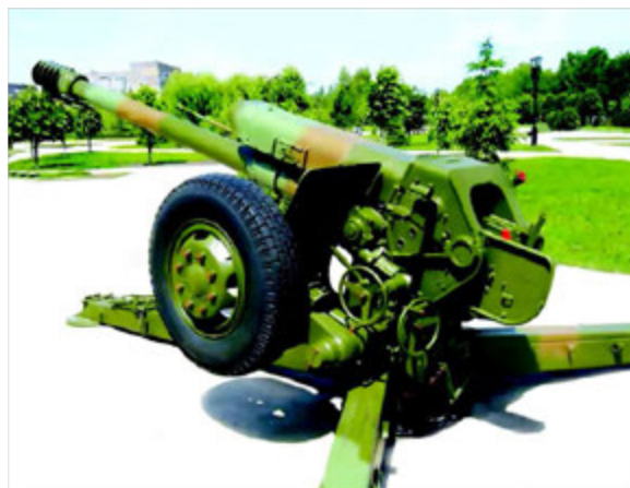
39-rasm. 122 mm.li D-30 zambaragi jangovar holatda.
