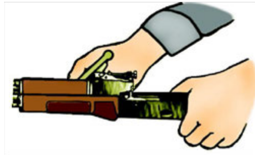
112-rasm. Gaz trubkasini stvol qo'ndog'idan ajratish.
